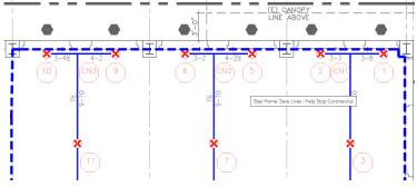
**Answer:** Sprinklers are required to be spaced 6 ft on center when protecting large openings or openings to stages per NFPA 13-2016 Section 8.15.4 and 8.15.17.2, respectively. In this case, a water curtain would not be required by those sections since there is no opening or stage-just a corridor.
